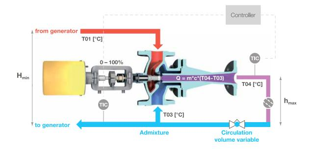
The primary differential pressure (Hmin) ensures the circulation of the required variable secondary water flow with the variable pressure drop (hmax) across the consumer.
