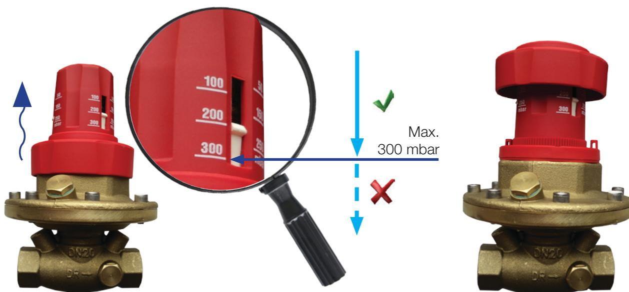
The differential pressure setpoint value is realised by lifting the red safety cap cover and turning the adjusting cap. The setpoint value setting required can be read off on the scale. Afterwards the safety cap cover is slid back towards the body. This fixes the setpoint value. It is also possible to fit a wire seal at the guide pins of the safety cap cover.
