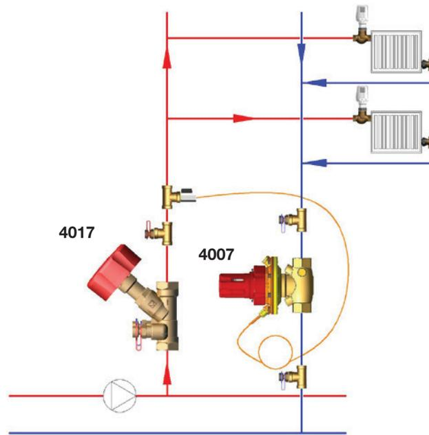
**Schematic 1: Differential Pressure Controller in the return**
