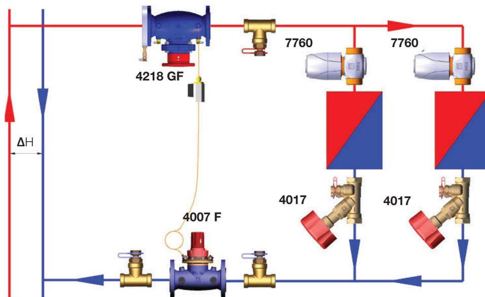
**Schematic 2: Differential Pressure Controller in the branch for the underfloor heating**
