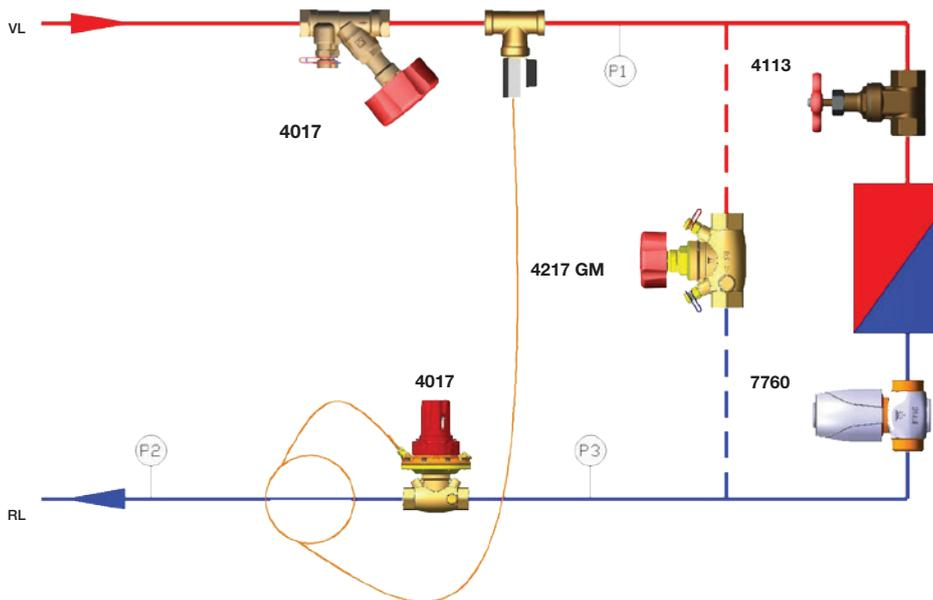
**Schematic 4: Commissioning the Differential Pressure Controller in an individual circuit**
