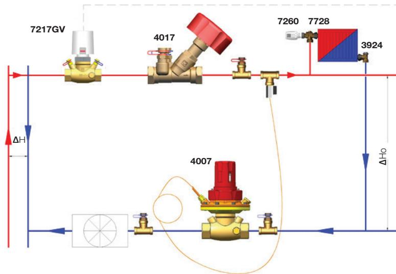
**Schematic 3: Control Valve in branch with Differential Pressure Controller**
